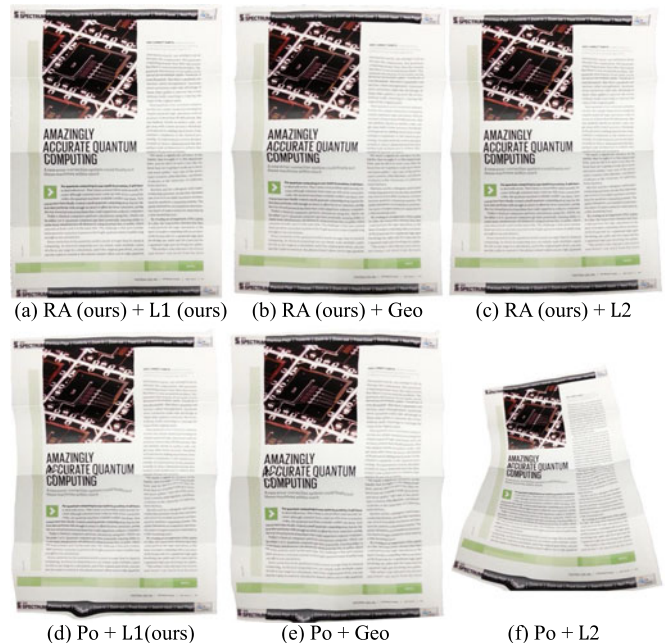
Fig. 5. Rectification results from combination of methods. Acronyms RA and Po denote our ridge-aware method and Poisson reconstruction respectively. L1 denotes our \ell_1 conformal mapping method with non-local constraints; L2 indicates LSCM [29] and Geo indicates geodesic unwrapping [30].
